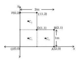
Find the centre of mass of uniform L-shaped lamina (a thin flat plate) with dimensions as shown in figure. The mass of lamina is 3kg.
